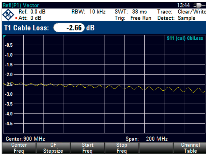
One-port cable loss measurement
