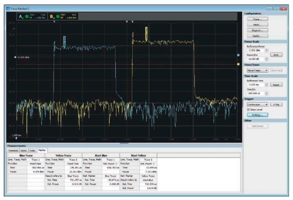
Pulse delay measurement on different traces
