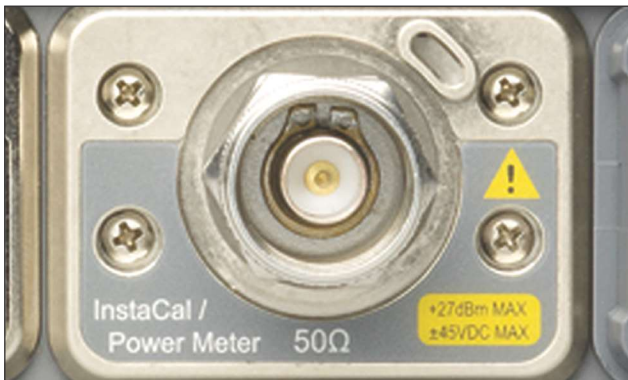
CLOSE UP VIEW OF INSTRUMENT TOP PANEL SHOWING INTERNAL INSTACAL MODULE
